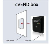
The cVEND box uses a similar concept as the cVEND plug, however the face of the unit is larger to compensate for mounting in a metal enclosure, positioning the antenna a sufficient distance away from the metal to maintain an outstanding reading performance.
